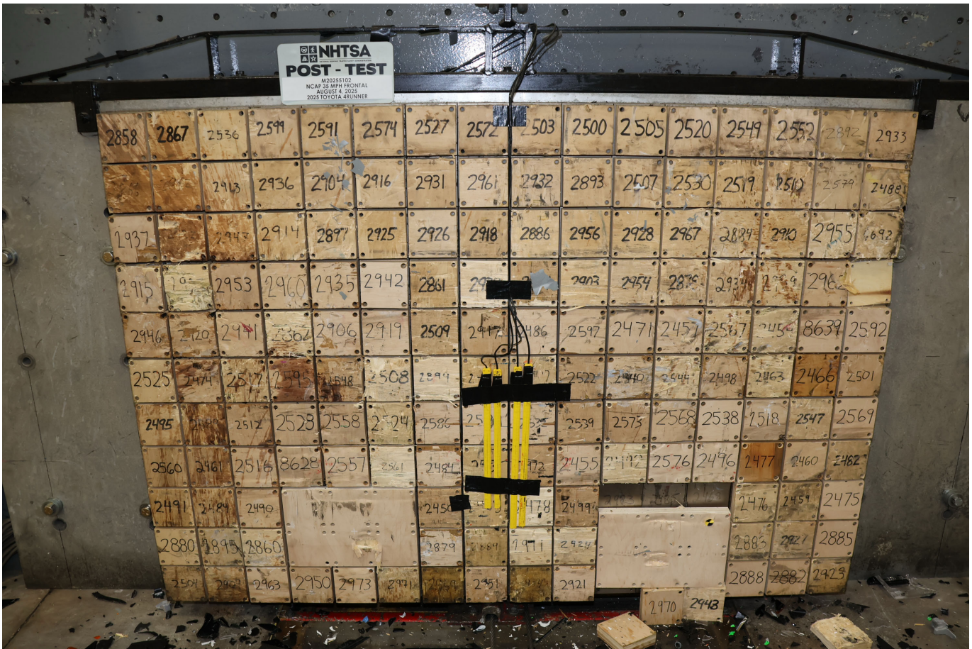
Photo No. 003 - Post-Test Load Cell Wall
