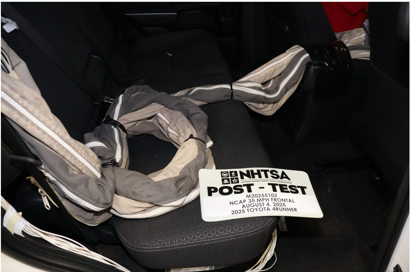
Photo No. 029 - Post-Test Dummy Cable Routing
