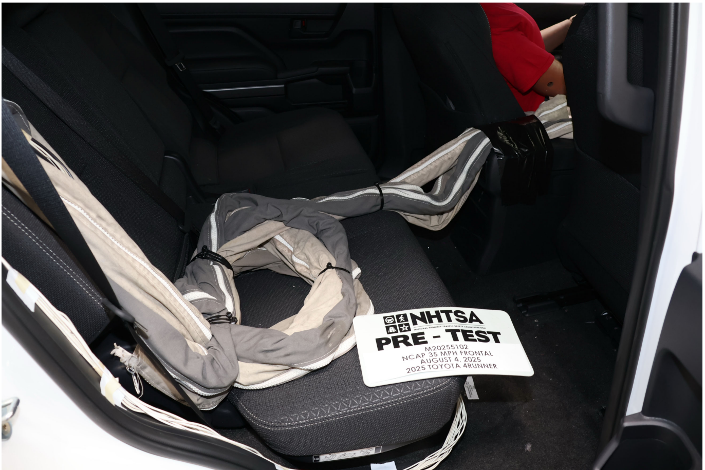
Photo No. 028 - Pre-Test Dummy Cable Routing
